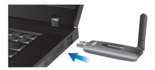
If using a Desktop PC, plug the Wireless USB Host Adapter into an available USB 2.0 port utilizing the provided extension cable.
